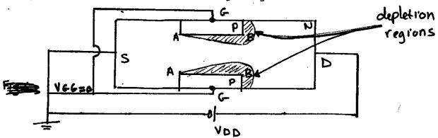
Since the P - layers are connected to zero voltage (ground) and because the layers are heavily doped, it follows that the voltages across the entire P regions are zero. Also, at the source end, the voltage is zero (because it is connected to ground). i.e. the net voltage drop across the PN Junction, at points A equal zero (thus the depletion layer is very small at these points.
