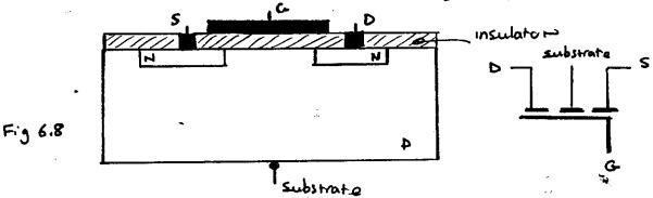
A P - substrate iused as the base substrate of the MOSFET. The Source and the Drain are connected , to two N - layers which are diffused on to the P - substrate . A metallic layer, deposited on the an insulating layer (called silicon dioxide), on the P - substrate and between the two N - layers is used as the gate of the MOSFET.
