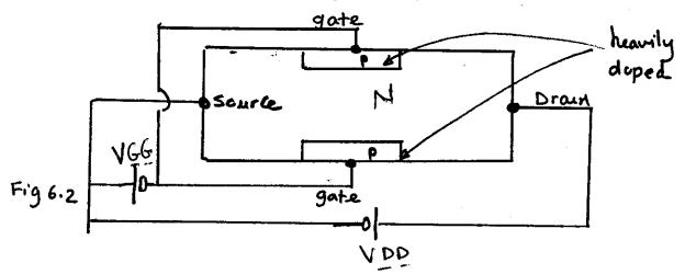
Let us first consider the operation of the JFET when  $V_{\text{GG}} = 0$  as shown in the following diagram :
