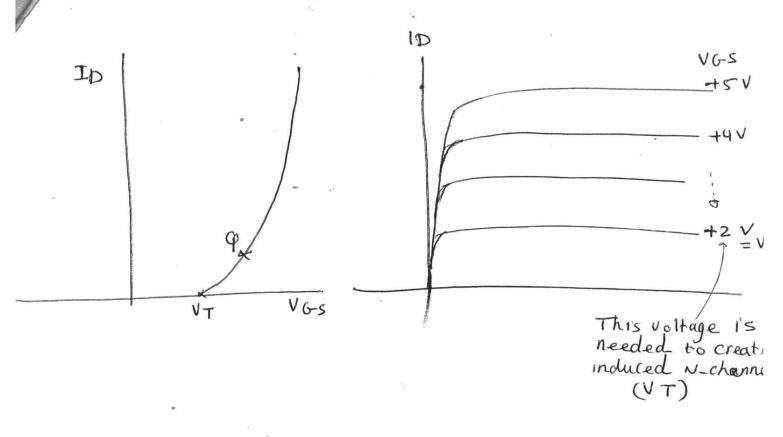
3- Brasing of ehancement FET should be made above VT (which is the critical gate voltage required to turn on the FET.)
