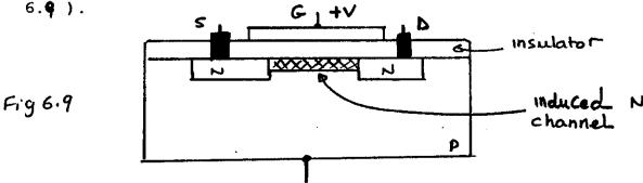
Under such condition and on applying a voltage  $V_{DS}$  across the Drain and Source terminals ,  $I_{D}$  starts to flow. Initially ,such current increases ,linearly ,with  $V_{DS}$  , up
