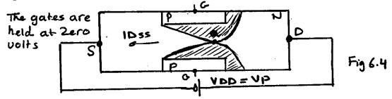
called , the saturation  $I_D$  or  $I_{DSS}$ , the saturation current (when  $V_{GS}$  is Short circuited ) which is determined by the developed potential at point a .
