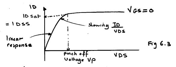
Eventually , a voltage  $V_{DS}$  is reached -- called the Pinch off voltage ,  $V_{P}$  -- where by the depletion layers touch each other at the middle of the N - Channel , as shown in Fig ( 6.4 ) , and the current  $I_{D}$  reaches a maximum value (
