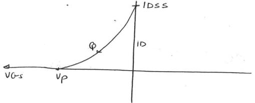
Note that if VGS is allowed to go positive, situation might arise where the gate/ource Junction becomes forward biased and urnent starts to flow between the gate and source
