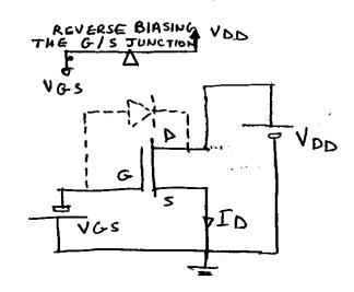
The depletion regions width can be increased (constricting the flow of current 10) by:
