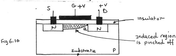
Any further increases in  $V_{DS}$  will not result in increases in  $I_D$  ( i.e.  $I_D$  reaches it's saturation value ). The following curves depicts the characteristic curves for this type of MOSFET device .
