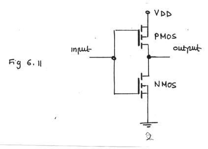
together to form a single input terminal . Also the two output source of PMOS and source of NMOS ( or source and drain ) are connected together to form a single output as shown in the above Fig .
