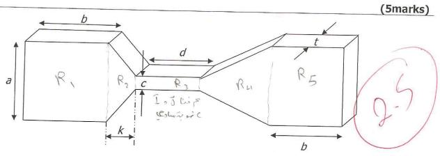
a = 4mm, b = 50mm, d = 20mm, k = 20mm, t = 0.1mm,  $\sigma = 5.7 \times 10^7 S_{100}$
